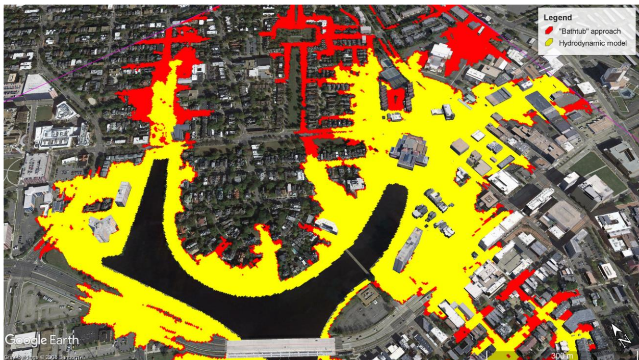
Fig. 17. Comparison between the storm surge model estimates for inundation extent under intermediate-high SLR in 2050 (yellow) and estimates based on the bathtub approach (red).
