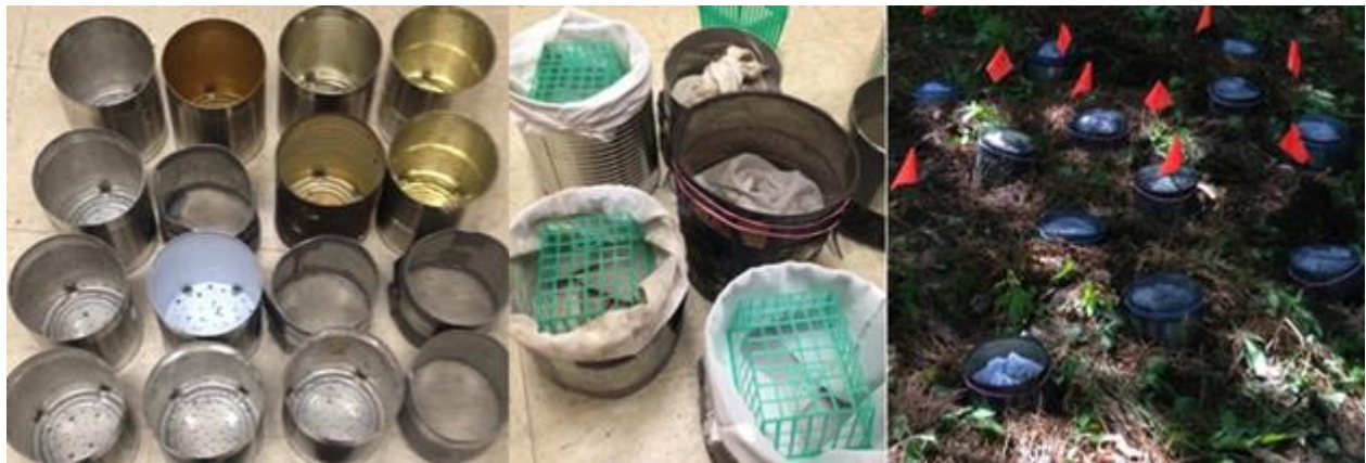
Fig. 6. Tickarium design empty (left), cloth bags, support baskets, and metal screen lids (middle), in situ tickaria (right); photographs taken by Lindsey A. Bidder on April 26, 2015 and May 2, 2015.
