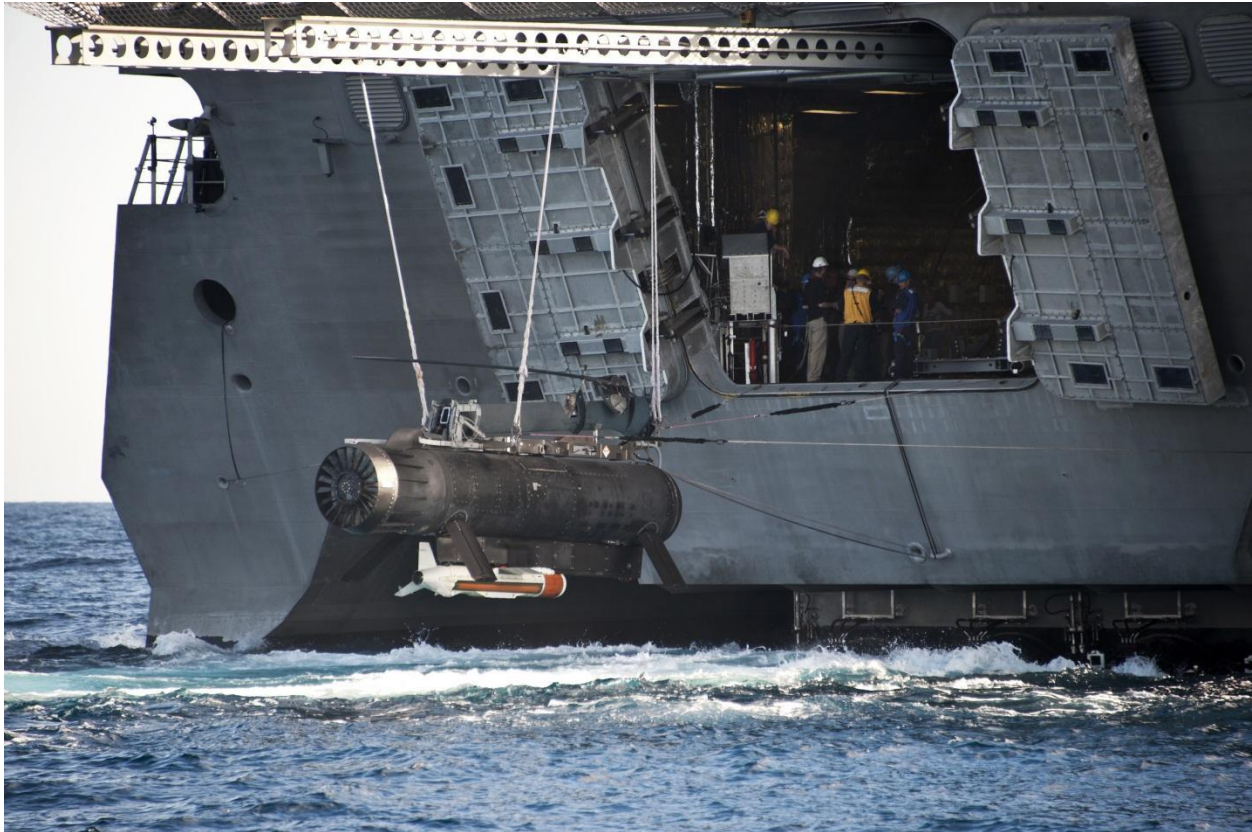
Figure 13- RMS recovery aboard LCS 2 387
