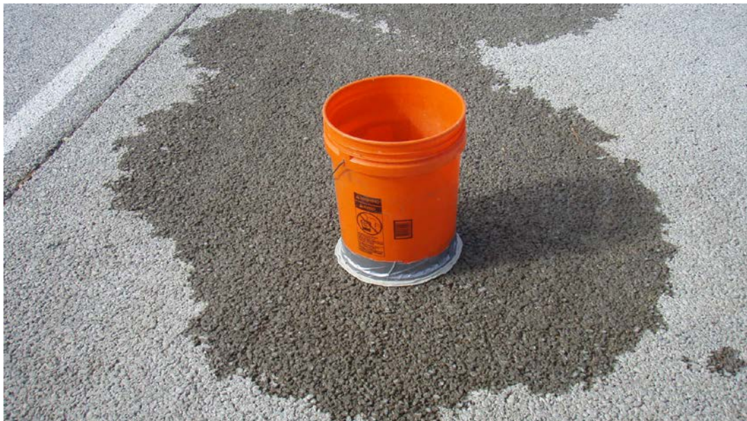
Figure 7. Extensive water plane flowing downhill on the surface of the pervious concrete away from the infiltrometer immediately after vacuum cleaning of pervious concrete at the Science Museum of Virginia on November 4, 2013.
