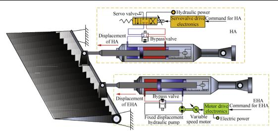
Fig. 1 Schematic of dual DRAS system.
