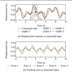
Fig. 8 Tracking responses when given superimposed sine-wave order using different FMPF based FTC.
