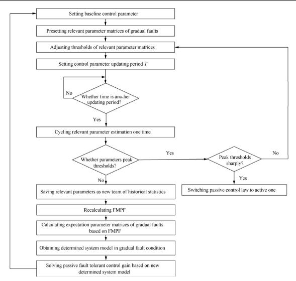
Fig. 3 Flowchart of FMPF based FTC mechanism.
