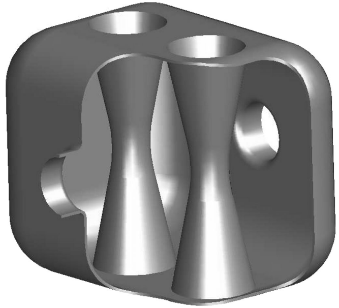
FIG. 16. Concept of a TEM deflecting structure with parallel bars of variable cross section.
