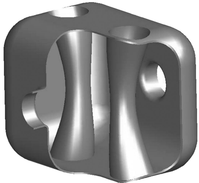
FIG. 17. Concept of a TEM deflecting structure with curved resonant bars.
