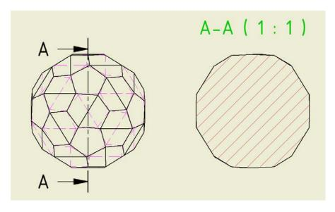
Figure 3. Triacontahedron Sectional View
