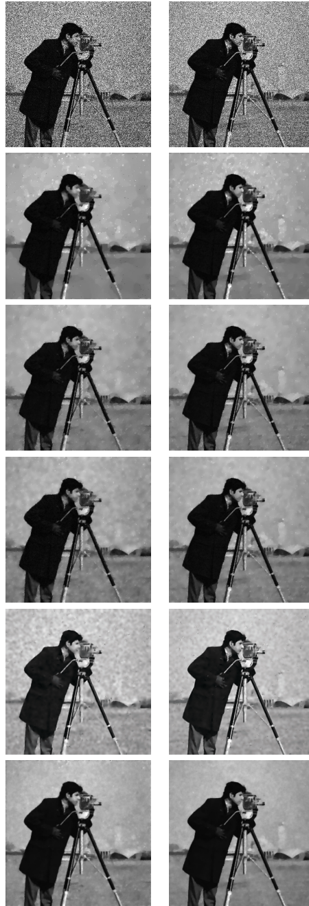
FIGURE 5. Results of various denoising methods on “Cameraman” image corrupted by multiplicative noise with L = 2 (the first column) and L = 4 (the second column). From top to bottom: Noisy images (8.63 dB, 11.64 dB), DZ (24.27 dB, 25.85 dB), TwL-4V (25.28 dB, 26.72dB), I-DIV (24.98 dB, 26.52 dB), HMNZ (25.30 dB, 27.33 dB), and Ours (25.47 dB, 27.38 dB).
