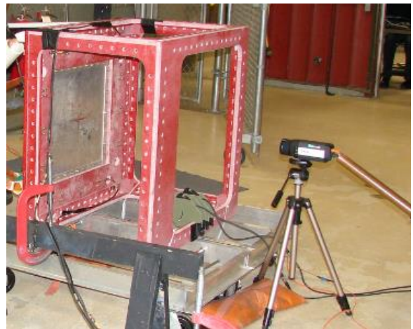
Fig. 10. Photograph of IR Camera used in test bed to capture backside temperatures at LTI.
