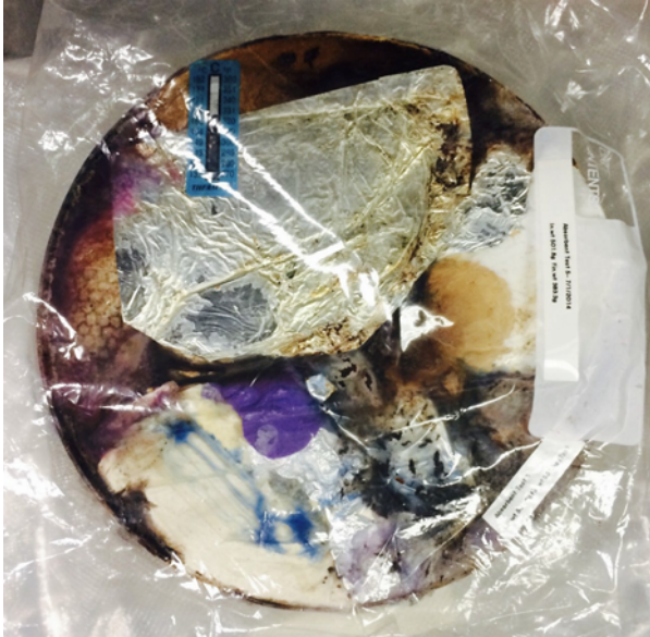
Figure 2. Photograph of Heat Melt Compactor tile tested at NSRL
