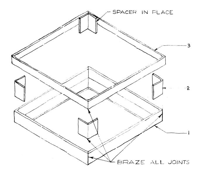
MATERIAL: PART NO.1 로HOT ROLL ANGLE IRON, STEEL PART NO.2 로HOT ROLL ANGLE IRON, STEEL PART NO.3 날 HOT ROLL BAND IRON, STEEL
