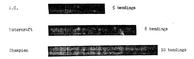
A linear graph showing point of spark plug ground electrode breaking expressed in number of breakings of ground electrode.
