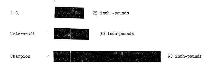
Linear graph showing pressure in inch-pounds at point of breakage of the spark plug center insulator.
