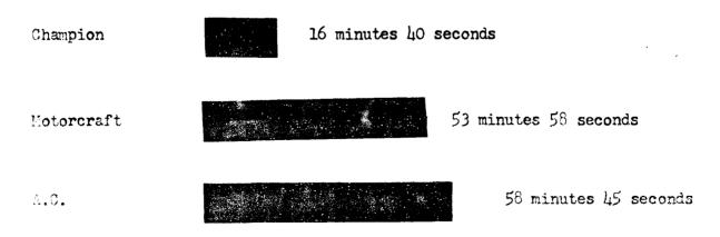
A linear graph showing the length of operation in minutes of Briggs and Stratton three horsepower engines before stoppage of engines due to oil fouling of the spark plugs.
