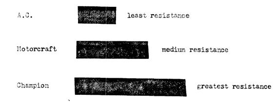
A linear graph showing hardness in resistance of center electrodes expressed in resistance.
