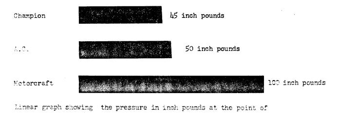
breakage of the spark plug porcelain insulator.
