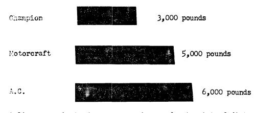
A linear graph showing pressure in pounds at point of distortion of spark plug shells.
