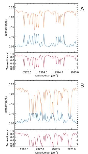
**Figure 2.** Emission correction for optically thin (A) and optically thick (B) lines of CH<sub>4</sub> at 700°C. The upper panels display the absorption (orange) and emission (blue) spectrum on the same arbitrary intensity scale; the lower panels display the transmittance (red).
