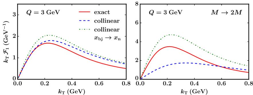
FIG. 6. Unintegrated structure function  $k_{\text{T}}\mathcal{F}_1$  for  $x_{\text{bj}} = 0.6$  and  $Q = 3$  GeV, with quark mass  $m_q = 0.3$  GeV and virtuality  $v = 0.5$  GeV for the exact result (solid red curves), approximate collinear approximation (dashed blue curves), and collinear result with the replacement  $x_{\text{bj}} \rightarrow x_n$  (dot-dashed green curves). The right-hand panel shows the results when the nucleon mass increased by a factor of 2.
