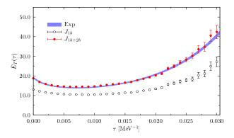
**Figure 2.** Euclidean electromagnetic transverse response function of  $^{12}$ C at q = 570 MeV (adapted from Ref. [18]). The theoretical predictions obtained including only one-body and both one- and two-body transition operators are represented by open circles and solid circles, respectively. The shaded band refers to the Euclidean response extracted from Ref. [19].
