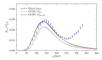
Figure 3. Electromagnetic transverse response functions of  $^4$ He at q=500 MeV. Experimental data are from Ref. [23].
