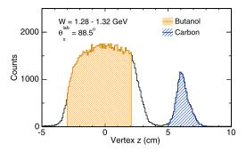
**Fig. 1.** Example of a reconstructed distribution of the reaction vertex along the beam line for events at  $W \approx 1.30$  GeV and  $\theta^{\rm lab} \approx 88.5^{\circ}$  originating in the butanol and carbon targets. The shaded areas indicate the *z*-vertex ranges used in the analysis.
