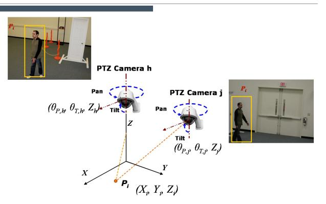
Figure 2. Typical setup of a pair of PTZ cameras
