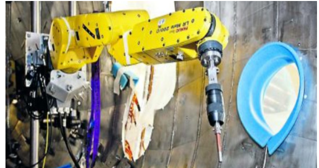
Figure 2 Fanuc LR Mate 200iC in a welding application
