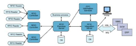
Fig. 3. Architecture of a RFID system [3]
