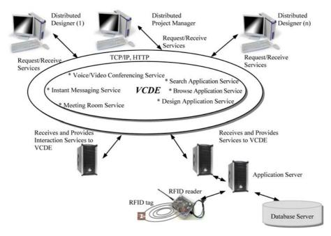
Fig. 1. DVCDGIE system architecture
