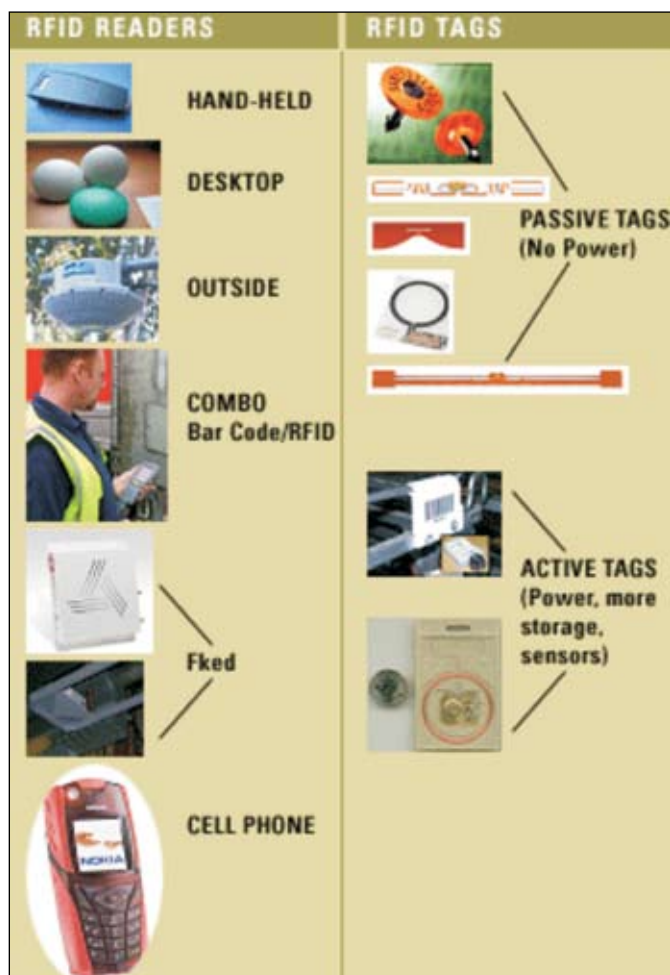
Figure 2. RFID readers and tags [2]
