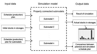
Figure 3. The Logical Scheme of the Simulation Model for Large-Scale Production
