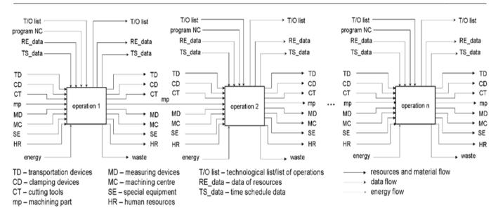
Figure 1. The Logical Scheme of the Simulation Model for a Unique Type of Production [7, 8]
