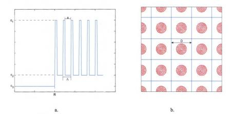
Fig. 1. scheme of the construction of the supercell square lattice of the Bragg fiber, (a) is the radial distribution of the dielectric constant and (b) is the supercell square lattice.
