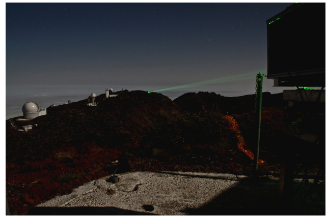
Fig. 3. The laser beam hits the mountain side about 500 m away from the transmitter during collimation tests to calibrate the beam size as a function of lens (L in Fig. 2a) position.
