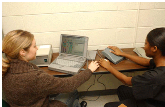
Figure 1 . Vibratory Sensory Analyzer (VSA) Showing Research Assistant on Left Measuring Tactile Sensitivity in a Subject.
