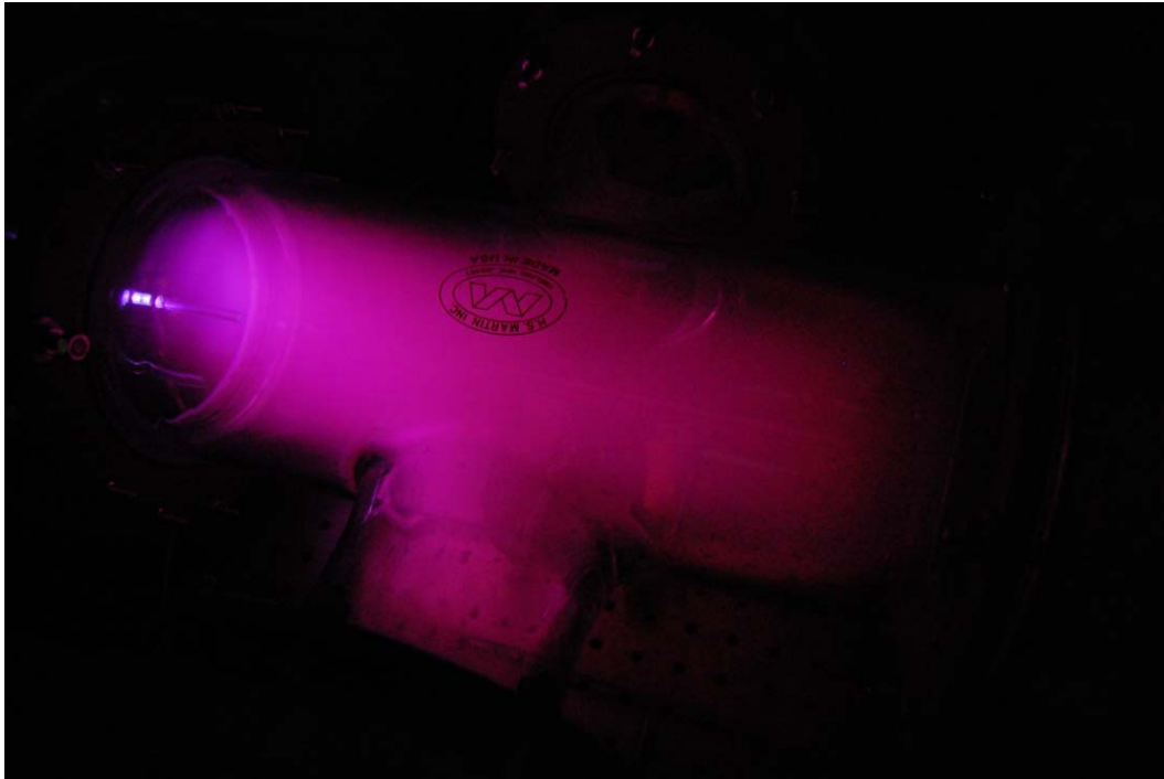
FIG. 8. Long exposure photograph showing a diffuse plasma filling the entire Pyrex chamber. The jet source (tube reactor) is visible to the far left.
