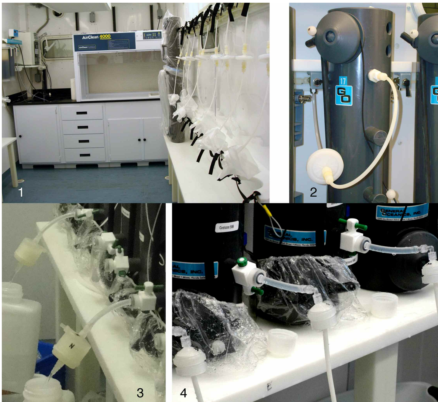
Fig. 2. Inside clean area of lab van and close-ups of GO-FLO air pressurization system, sampling with capsule filters, and sampling with membrane filters.
