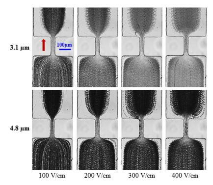
FIG. 5. Superimposed images illustrating the electrokinetic focusing of  $3.1 \,\mu\text{m}$  and  $4.8 \,\mu\text{m}$ -diameter particles (the images for 9.9  $\mu\text{m}$  particles are referred to Fig. 1) in 200 ppm PEO solution under four different DC electric fields. The block arrow indicates the particle moving direction in all images.
