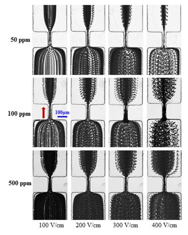
FIG. 4. Superimposed images illustrating the electrokinetic focusing of 10  $\mu$ m-diameter particles in PEO solutions of various concentrations (0 and 200 ppm are referred to Fig. 1) under four different DC electric fields. The block arrow indicates the particle moving direction in all images.
