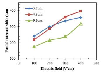
FIG. 6. Experimentally measured stream widths of the electrokinetically focused particles with different sizes in 200 ppm PEO solution in the constricted microchannel. The unfilled symbol for 9.9  $\mu$ m particles represents the point at which particle aggregation inside the constriction was observed. The particle stream width of this point is obtained from the superimposed images prior to the occurrence of particle aggregation.
