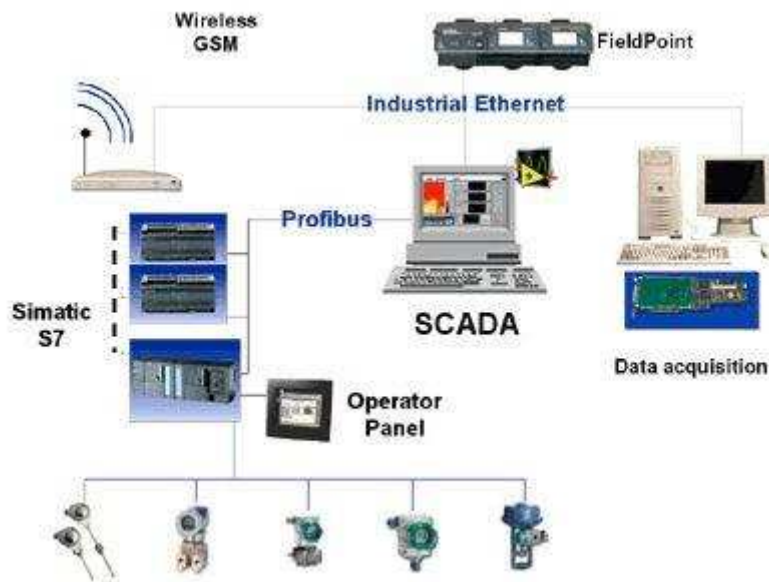
Figure 1. Supervisory Control and Data Acquisition
