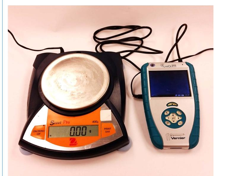
Figure 4. Talking Labquest and balance for determining mass audibly.
