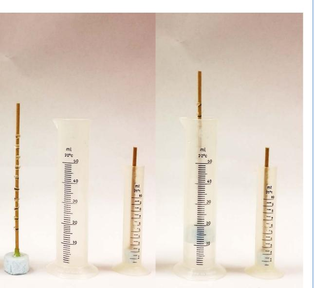
Figure 5. Graduated cylinders with floats for determining volumes of non-volatile solvents.
