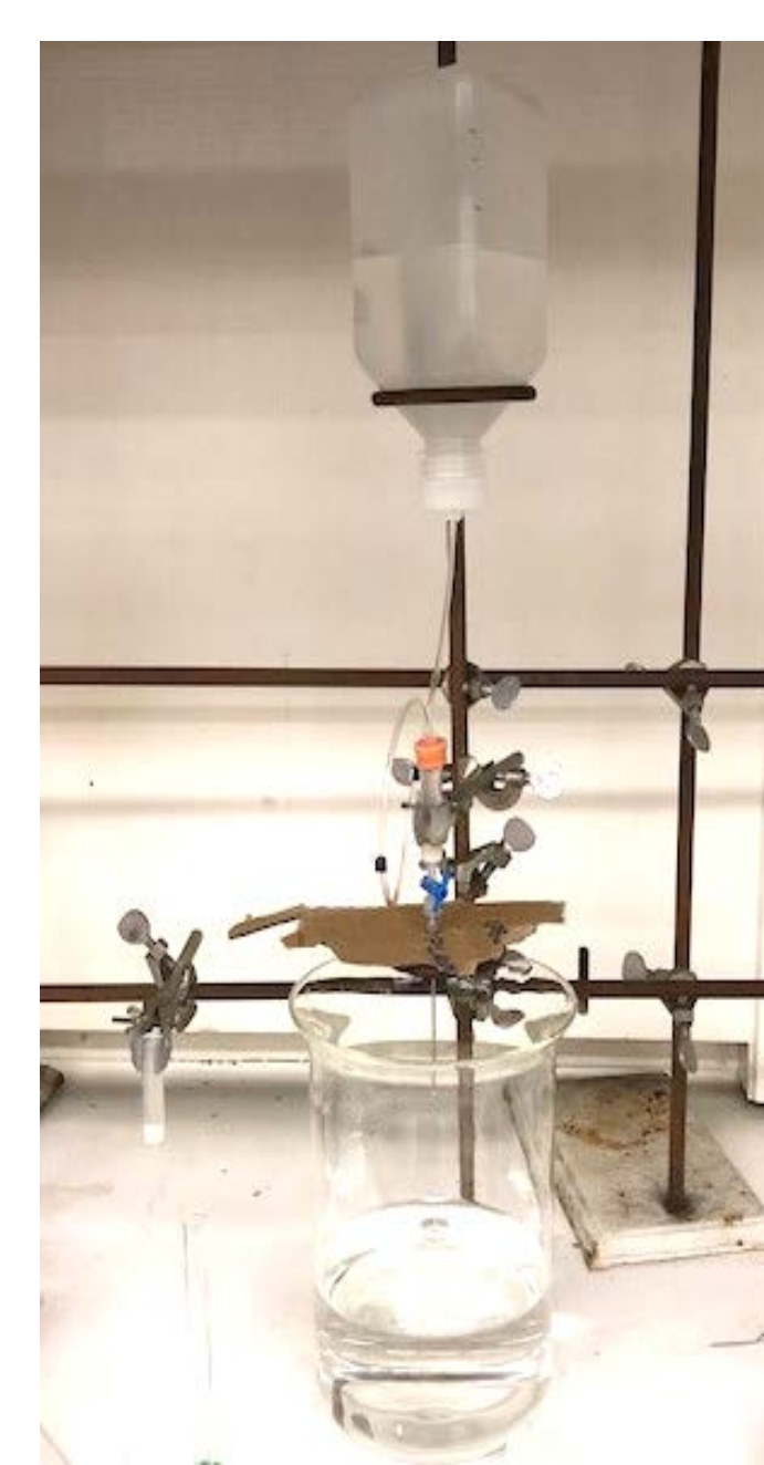
Figure 3. Extraction set-up for sample solutions
