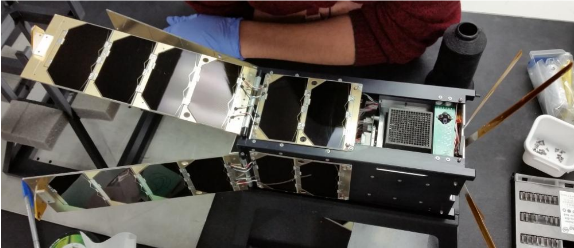
Figure 4.2.1-5: Solar panels are attached
