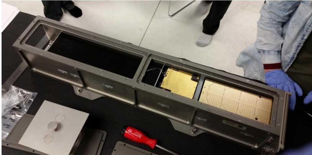
Figure 5.1-4: Satellites integrated into NRCSD prior to vibrational testing
