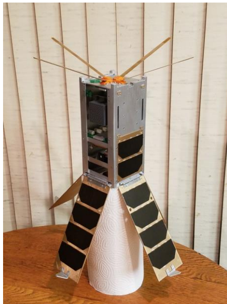
Figure 3.3 Fully 3D printed CXBN-2 model
