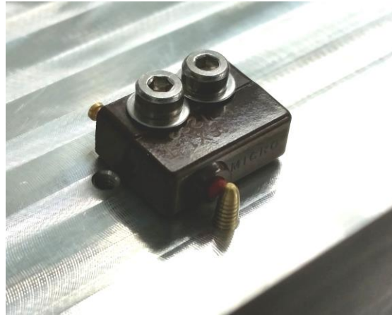
Figure 3.5.5-3: RBF pin and switch
