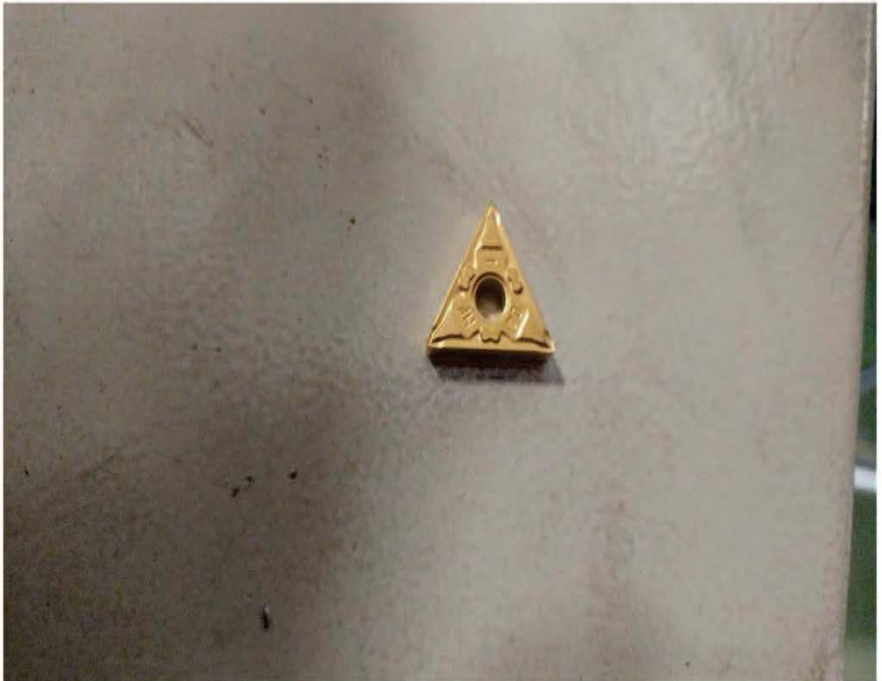
Figure 3.18: Finishing Insert: Sharper Nose
