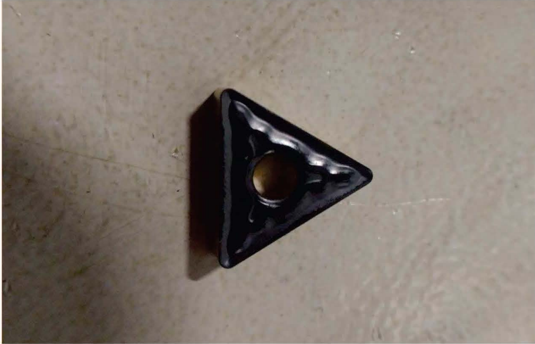
Figure 3.19: Roughing Insert: Rounded Nose
