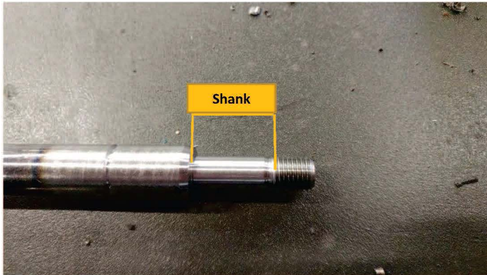
Figure 3.21: Piston End Shank
