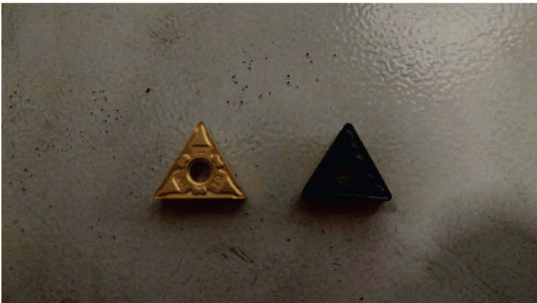
Figure 3.17: Inserts: Finishing (Left) and Roughing (Right)
