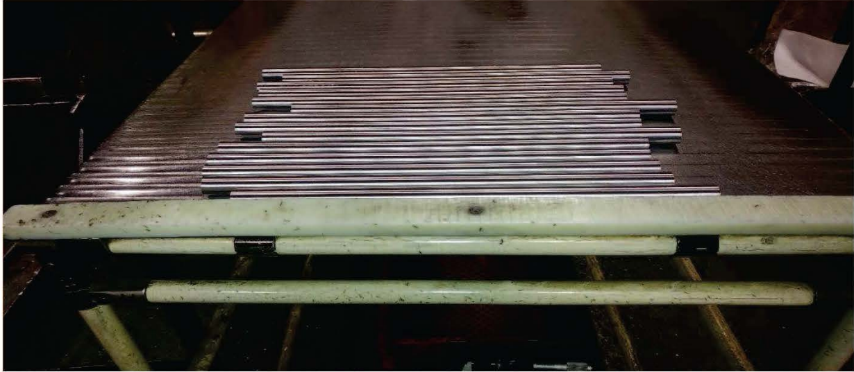
Figure 3.5: Completed pre-grinder rods
