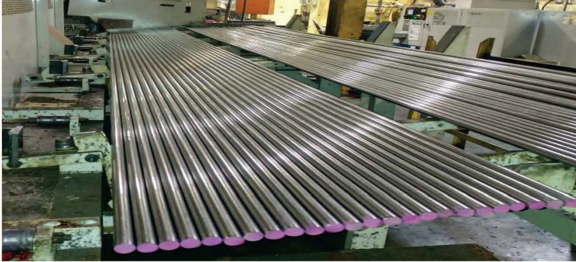
Figure 3.2: Rods sent through a machine to be cut at 395 mm length
