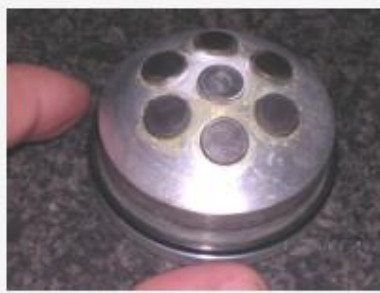
Figure 1 metal-bonded diamond pellets on hard tool
