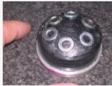
Figure 5 stainless steel washers on 40mm bonnet
