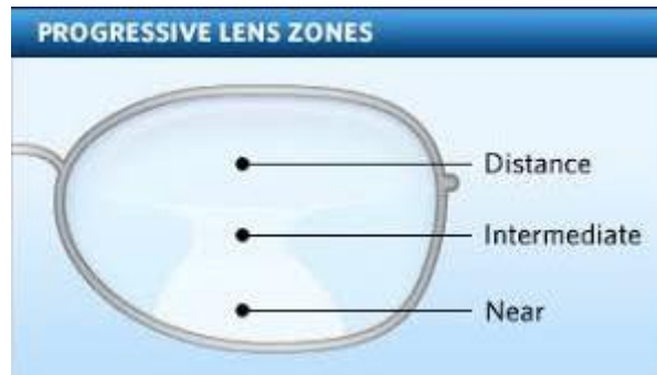
Figure 2-13: Progressive lens zones [107]
