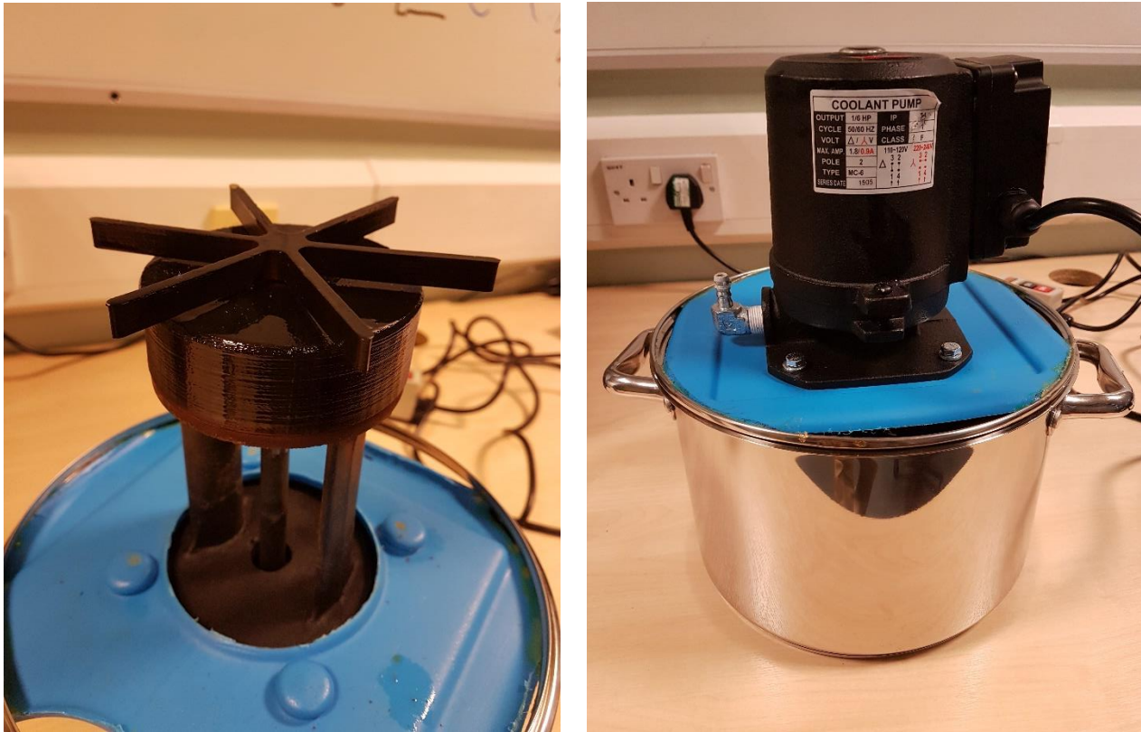
Figure 4-20: 3D printed pump cover on left and slurry tank on the right
