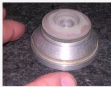
Figure 2 resin-bonded diamond hard ring tool
