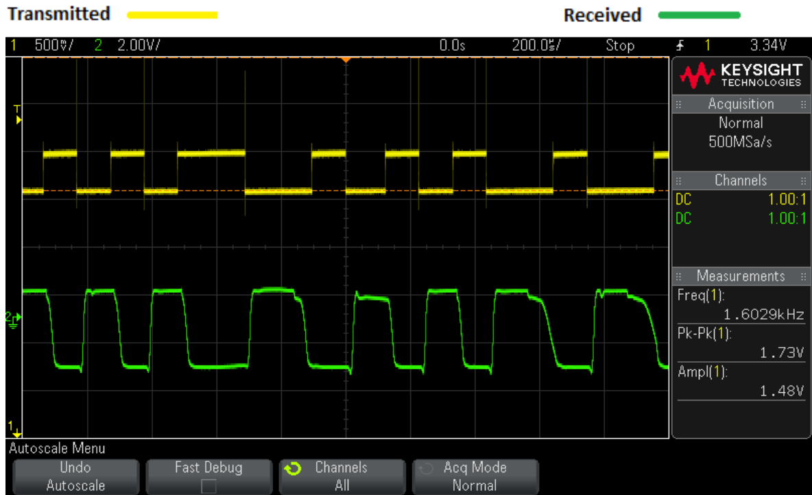
Figure 6.9 Signal captured at the output of MFB filter distance of 150cm
