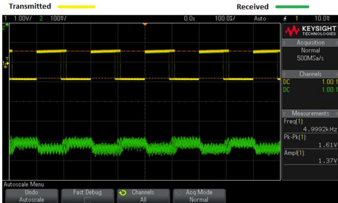
Figure 5.4 TIA output signal without filtering distance of 1.5m
