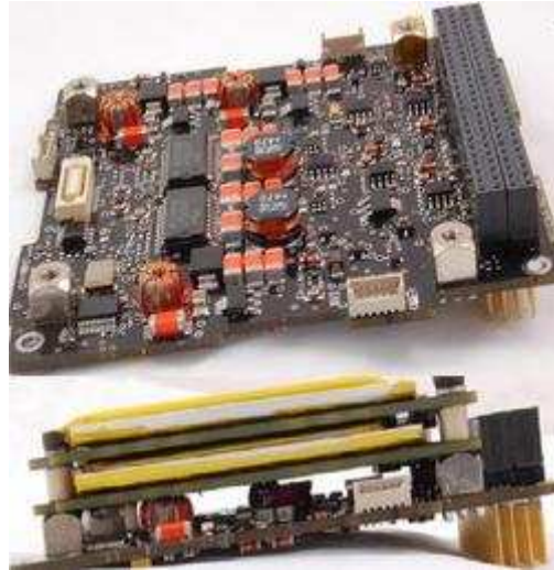
Figure 2.2: Clyde Space 1-U CubeSat EPS board (CS-1UEPS2-NB). This revision was similar to the EPS flown on KYSat-1. The board on the bottom demonstrates the EPS integrated with lithium-polymer battery cells.
