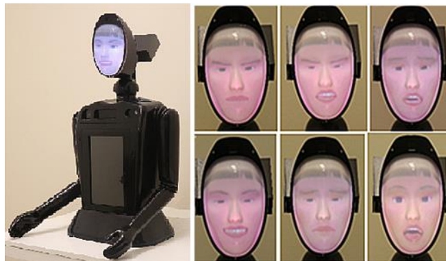
Figure 1. Left) Ryan Companionbot robot [31,32]. Right) Expressions demonstrated by Ryan with 100% intensity (Top from left to right: anger, disgust, fear. Bottom from left to right: happiness, sadness, surprise)
