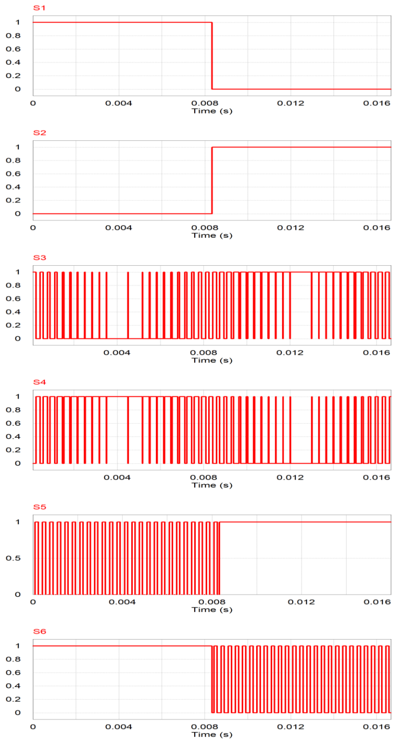
Figure 4. 10 Modulation strategy of H6 topology
