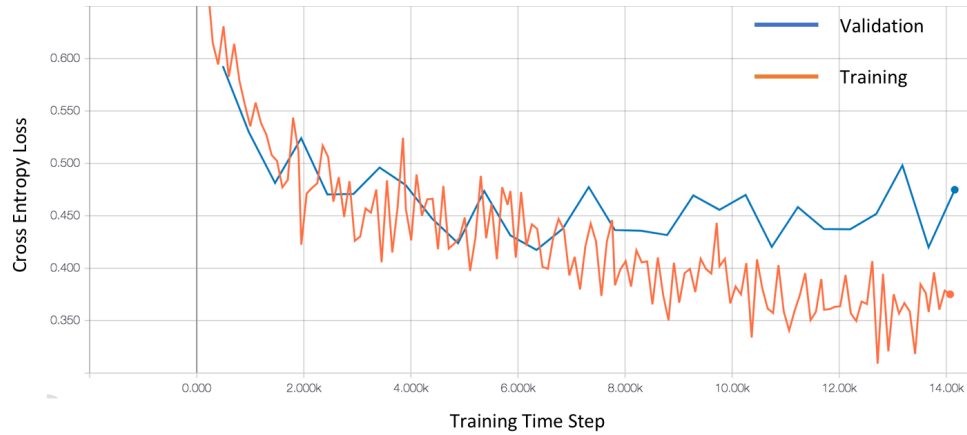
Figure 3.3: Cross entropy loss curve of the BE model from start to the end of the training. Figure shows validation and the training loss. The best model was obtained at 6,834 steps which is approximately 6 epochs
