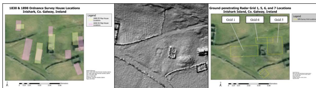
Figure 7: A comparison of building locations on 1838 and 1898 Ordnance Survey maps (left) and LiDAR map data (center) helped select ground-penetrating radar (GPR) survey grid locations. The locations of GPR survey grids 1, 5, and 6 are shown on the modern landscape (right). Maps produced by author in ArcGIS Pro.
