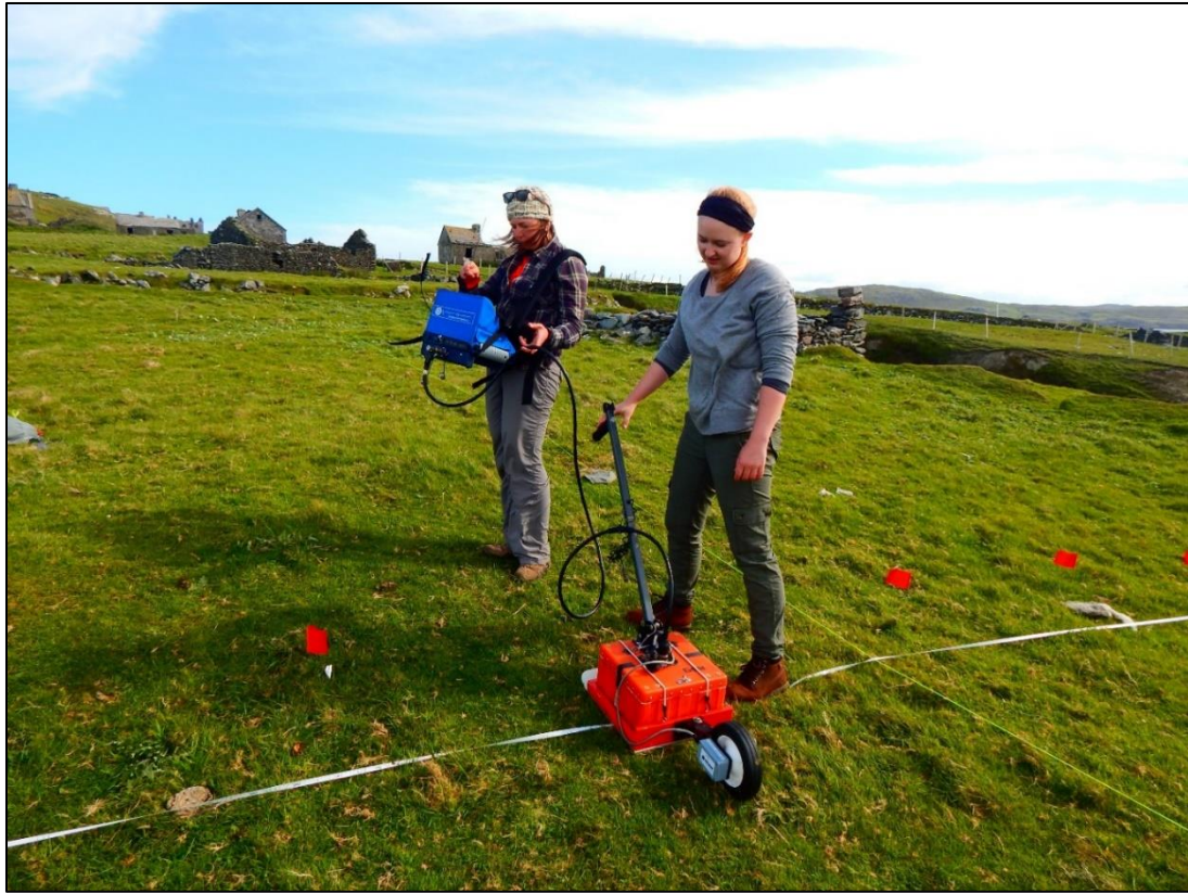
Figure 4: Ground-penetrating radar (GPR) 400mHz antenna connected to a survey wheel, which measures distance. Personal photograph.
