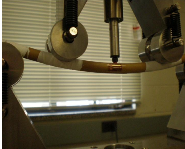
Figure 3.2: 4 point loading configuration with modified saddled loading pins and Teflon ® tape at points of contact.
