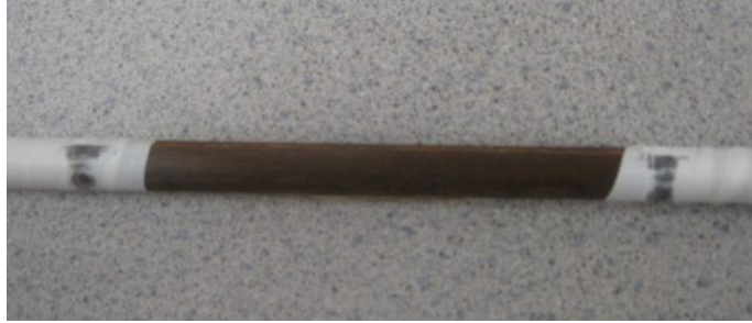
Figure 6.6: Surface damage of a specimen aged at 180°C for three months.
