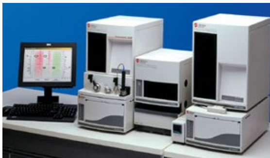
Figure 6 - Eprogen ProteoSep™ multidimensional high-performance liquid chromatography system. System uses two dimensions of separation (chromatofocusing and reverse-phase chromatography) to separate entire proteomes from a single injection.
