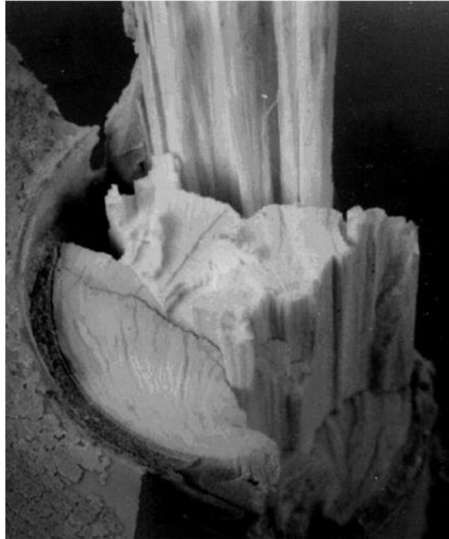
Figure 2: Brittle Fracture of a 500 kV Composite Insulator
