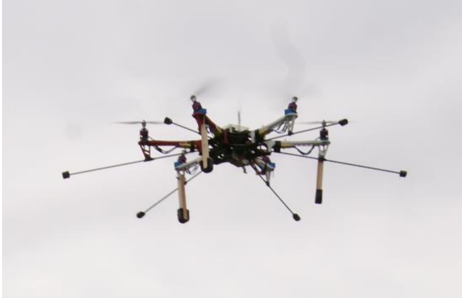
Fig. 2.3 The Dexterous Hexrotor, note the rotors are nonparallel.
