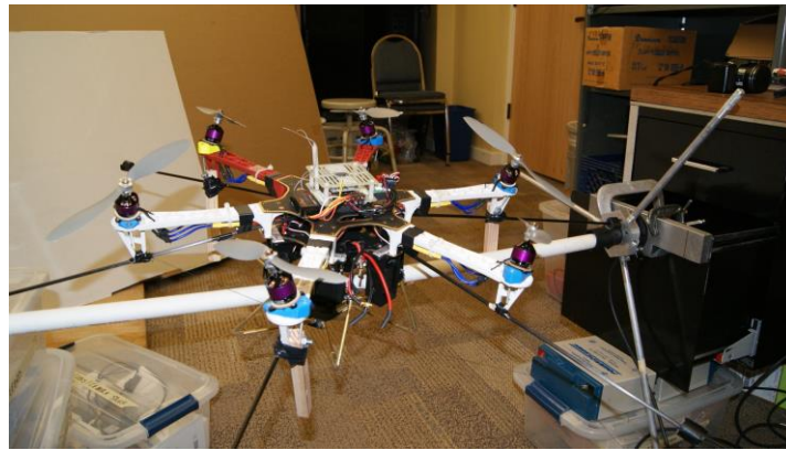
Fig.5.6 Peg-in-hole setup with the Dexterous Hexrotor.
