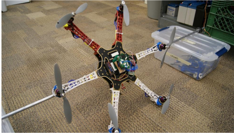
Fig.5.3 PID controller test set up
