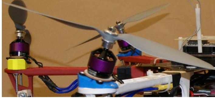
Fig. 4.2 Motor mounted on a 20° ABS plastic adapter
