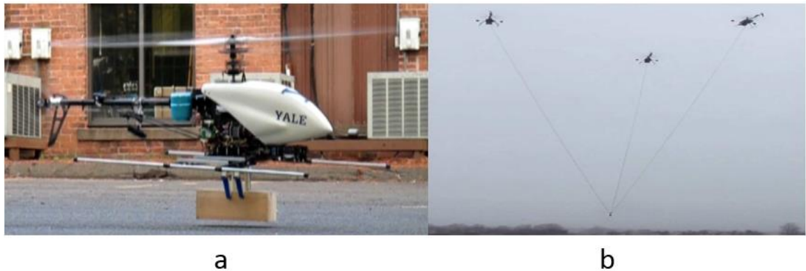
Fig. 1.4 Aerial Mobile Manipulation: (a) Yale Aerial Manipulator capturing a block in hover (Three helicopters transporting a load (Reprinted with permission from Paul E.I. Pounds and Ivan Maza)
