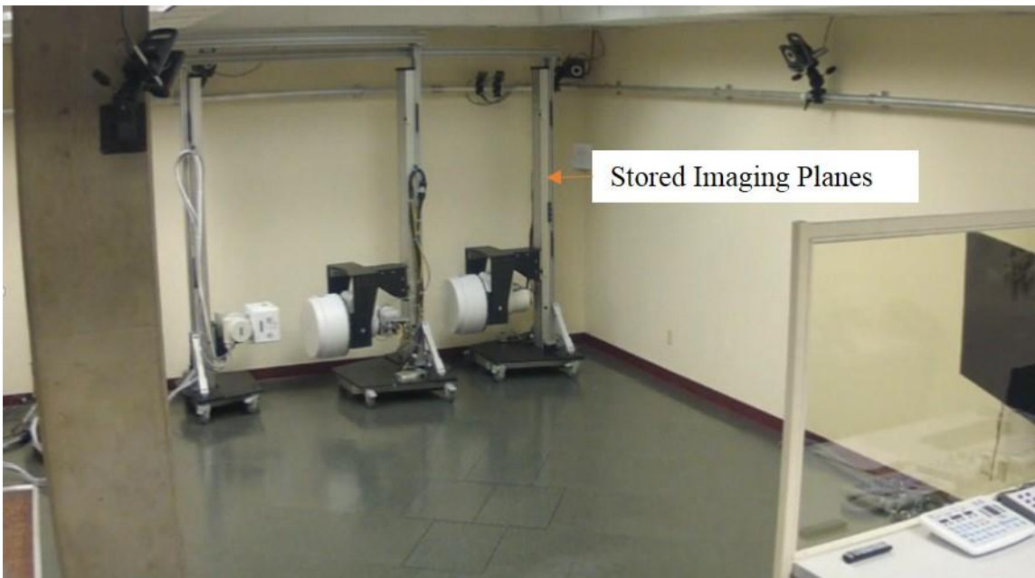
Figure 2-7: The stored imaging planes are aligned against the wall.
