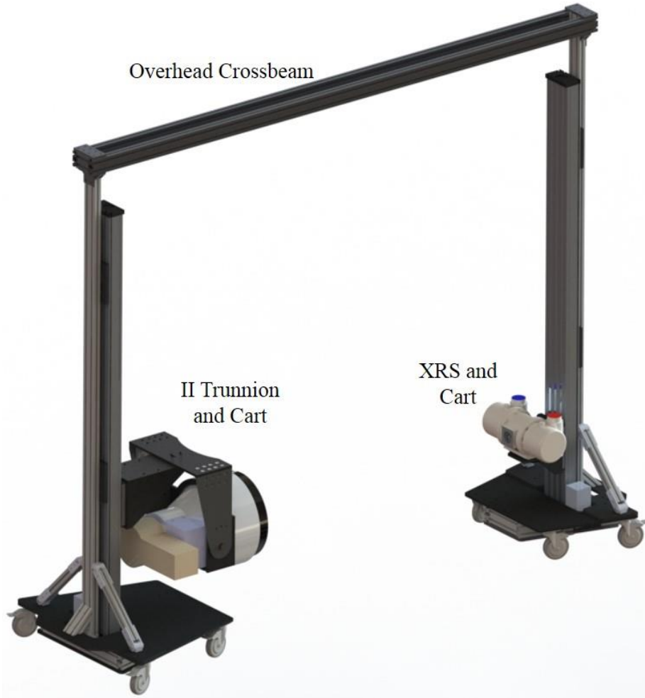
Figure 3-29: The completed plane consisting of an II trunnion, an XRSS, their respected carts and an overhead crossbeam to tie them together.
