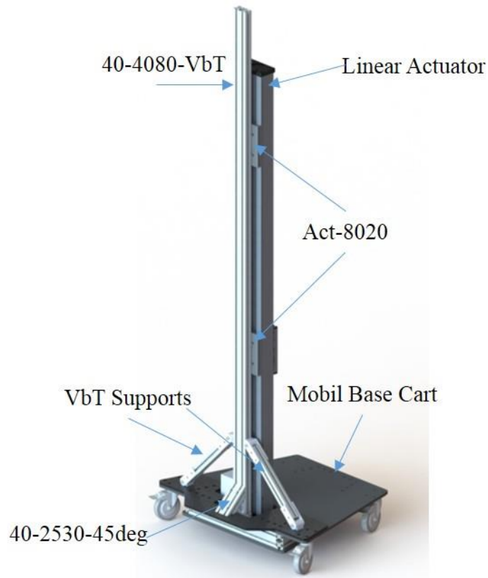
Figure 2-2: The II cart with all the pieces between the overhead crossbeam structure and the base cart, labeled. The II and trunnion are hidden in this picture.
