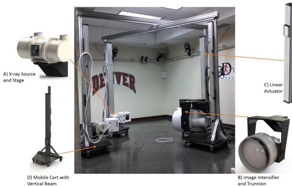
Figure 2-1: The HSSR system comprised of the following sub-systems: (A) X-ray source, (B) image intensifier, (C) linear actuators, and (D) mobile cart and vertical beam.
