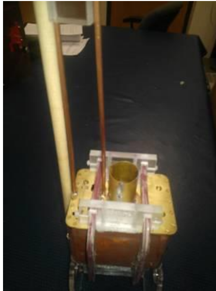
Figure 7.12 CLR-CH-2 as of March 2014. The power resonator is two coils of 0.1 mm diameter wire, 52 mm in diameter and spaced 38 mm in. Detection resonator is a single turn resonator, 26 mm in diameter and consists of 25 parallel coils of 0.1 mm diameter wire spaced about 1.3 mm.
