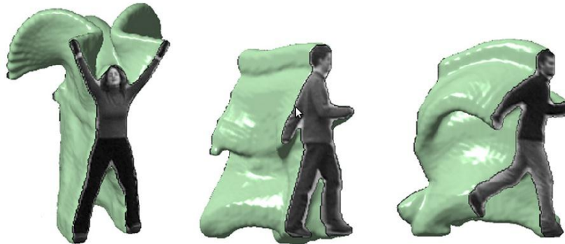
Figure 2.3. Space-time volumes for action recognition based on silhouette information (Blank et al. [3])
