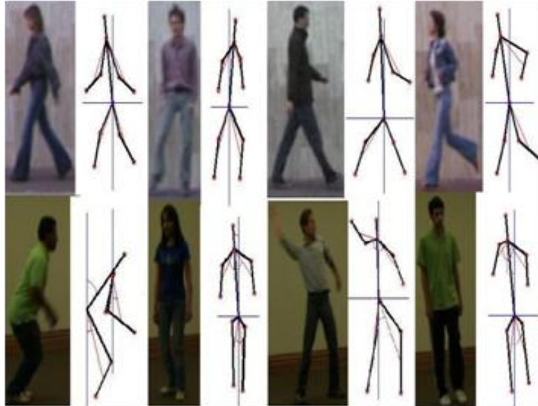
Figure 4.6. Each frame shows the five angles that provide orientation data of torso and limbs.
