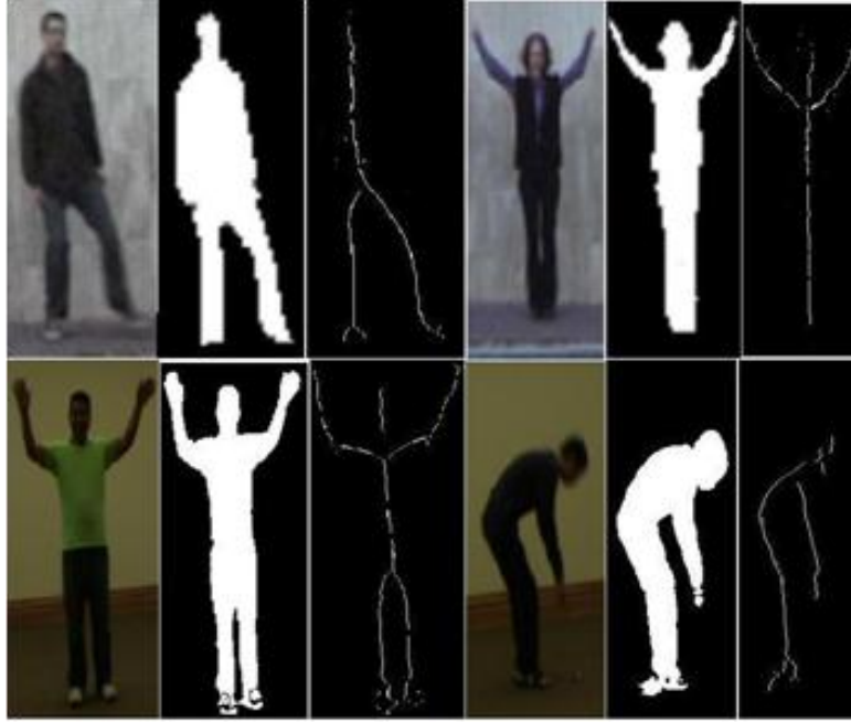
Figure 4.3. Illustrates the results of background subtraction and skeleton extraction using MAT algorithm.
