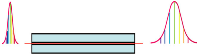
Figure 2.14. effect of dispersion on an optical pulse in a fiber link
