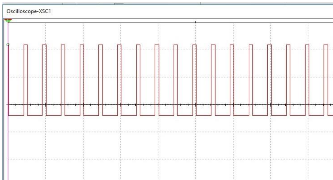
Figure 4.11: Switching signal output
