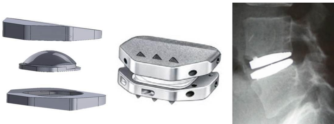
Figure 2.3 The Aesculap Activ-L consists of a titanium superior end plate, UHMWPE inlay, and a titanium inferior end plate. The inlay is free to translate in the anterior-posterior direction within the inferior end plate. Exploded view (left) assembly (center) after insertion into FSU (right)( www.fda.gov ).
