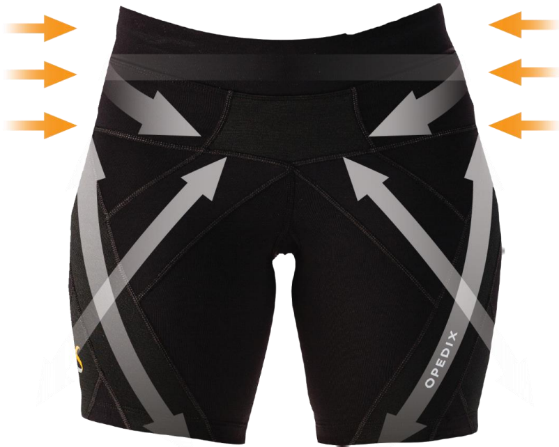
Figure 3.1: The CoreTec short (Opedix LLC, USA) with arrows indicating the design providing directional compression that replicates the function of the hip abductor muscles with diagonal bands of fabric with low elasticity spiraling downwards from the waist and hips to the thighs. This banding pattern is overlaid onto a standard compression base layer with high elasticity and is designed to facilitate neuromuscular control of pelvic orientation, hip adduction, and hip external rotation.
