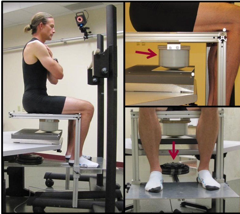
Figure 3.2: Unstable sitting experimental setup (left). A chair was affixed over an adjustable hemisphere (top right) while an adjustable 12-kg counter weight was attached to the foot plate of the chair (bottom right) to offset the mass of the feet and legs.
